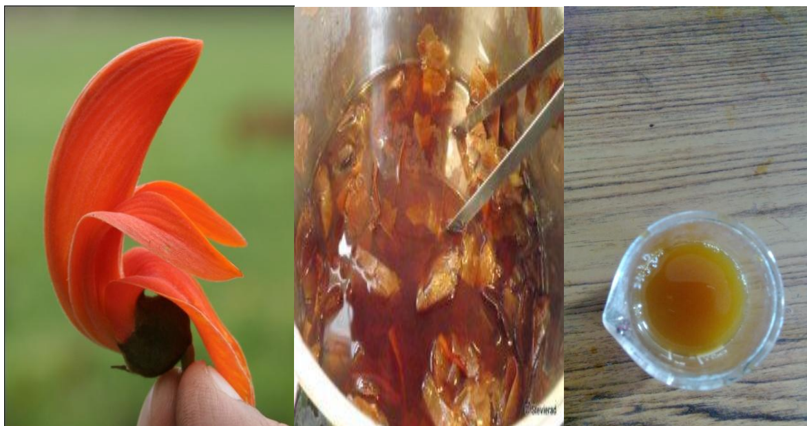
Figure 2. Extraction of Dye From Butea Monosperma (Daberao, et al., 2016)
